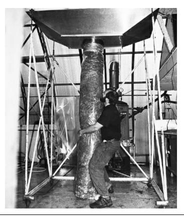
When the column is slammed to the floor during filling, the straw packs densely.
