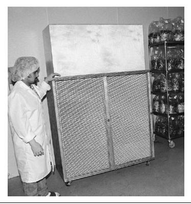
A portable laminar flow wall creates a localized clean zone in which newly autoclaved substrate can safely cool without danger of contamination.
