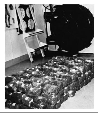
Three times the formula featured earlier in this chapter created 210 6-pound (< 3 kg) bags of the fruiting formula. Once mixed and wetted, this mixture must be immediately loaded into the autoclave and sterilized.
