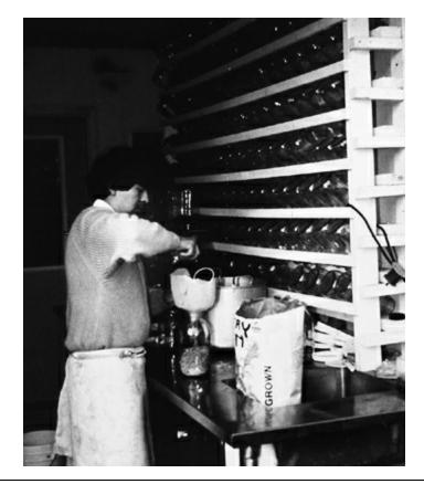
One method for preparing grain spawn is to simply pour dry grain into glass jars, then add water, allow to sit overnight, and then sterilize. Advantages are a one-step process, less fuel consumption, and less handling. One disadvantage is uneven water absorption.
