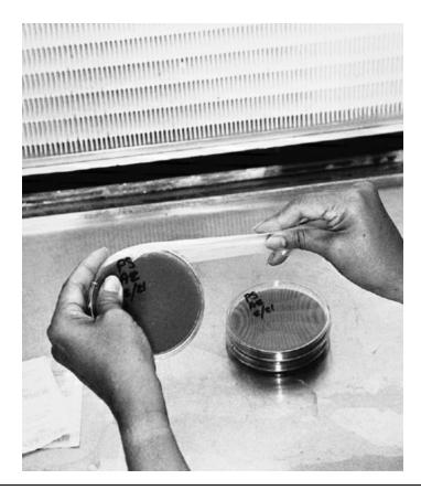
Using an elastic film to seal the top and bottom of petri dishes. This eliminates the chance of airborne contamination entering during incubation.
