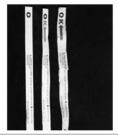
Heat-sensitive sterilization indicator strips showing no sterilization, partial sterilization, and complete sterilization.
