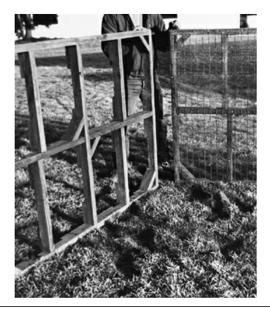
Screened floor racks allow the passage of steam underneath the bulk material being pasteurized.
