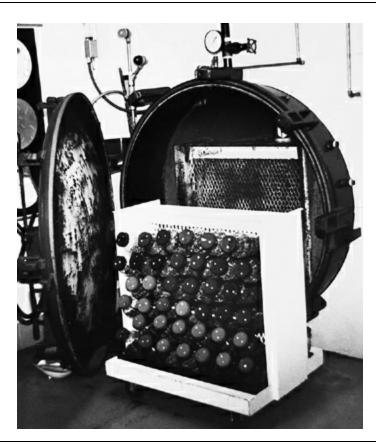
Grain-filled <sup>1</sup>/<sub>2</sub>-gallon jars ready for loading into a commercial autoclave.
