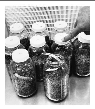
Sterilization indicator test strips are placed into a few grain-filled jars to test sterilization. Note the letter "K" appears when sterilization has been achieved.
